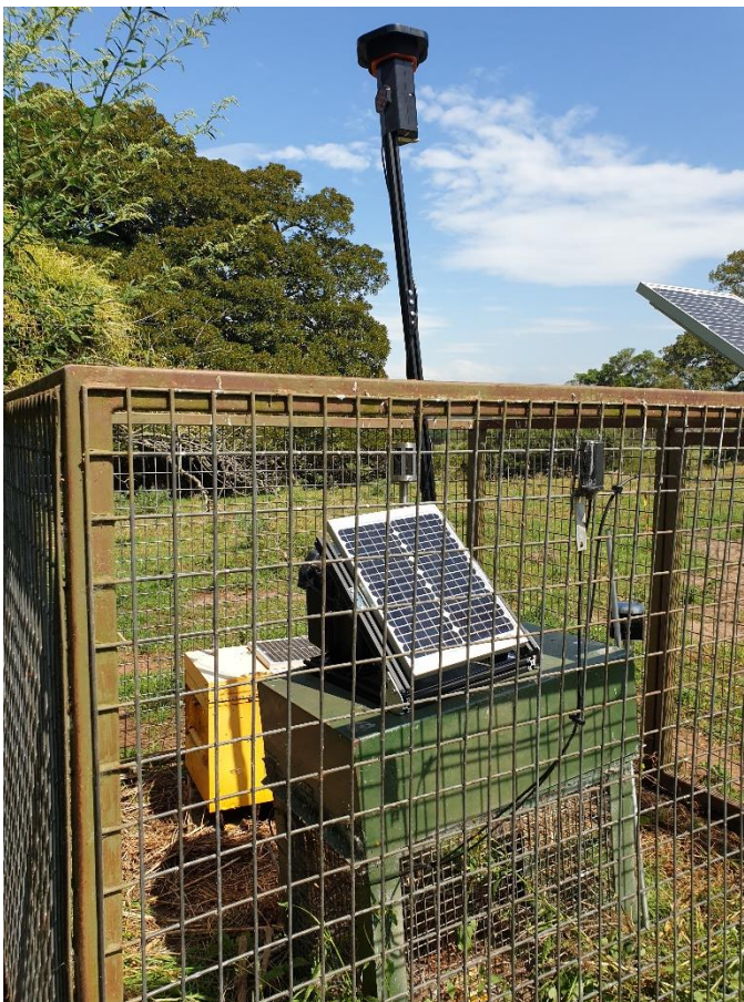
Figure 2 Real time noise monitor established near the Figtree Hill residences. Blast monitor also in compound.
