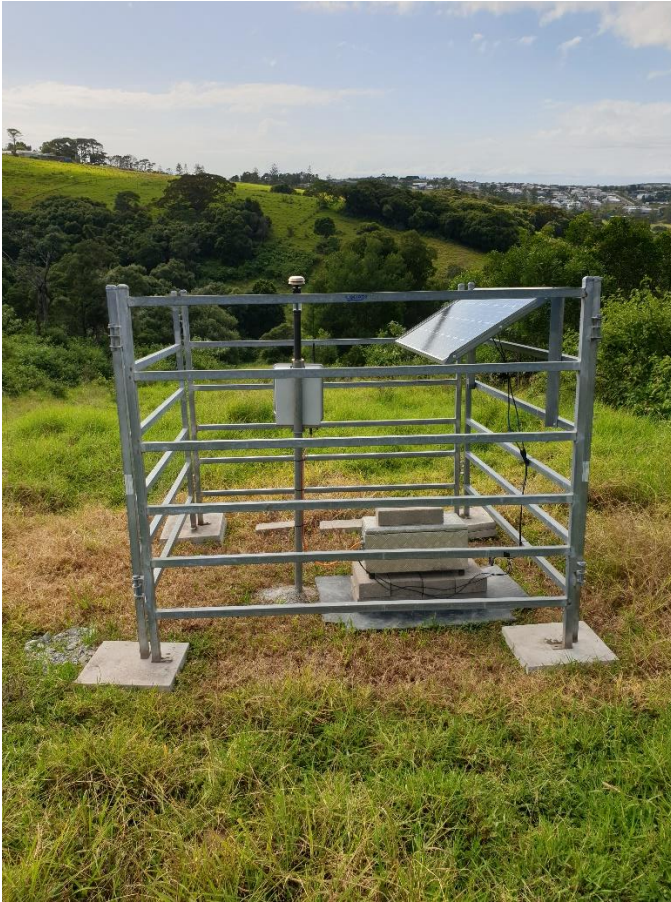
Figure 1 Real time particulate dust monitor established east of Stage 7 area.
